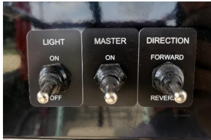
Control switches for light port, master, and direction. (LED light is not included in base model)
